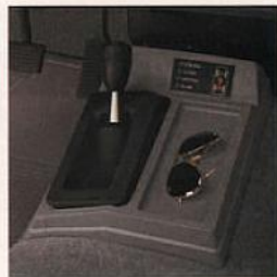
Insta-Trac transfer case provides shift-on-the-fly convenience.
